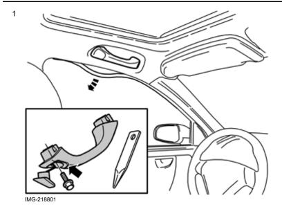
Carefully prize up the top edge of the cover where the glasses holder shall be located. Use a plastic weatherstrip tool.
