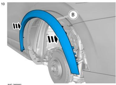
Install component that comes with the accessory kit. Ensure that all clips engage.
