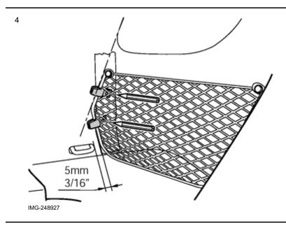
Press two clips into the rear end of the net pocket. The buttons (1) of the net pocket must be facing outwards.
