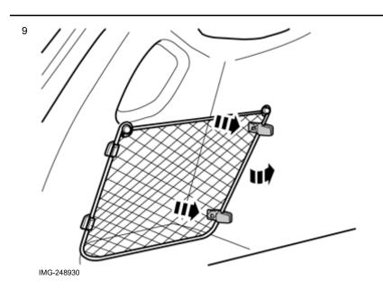
10 30mm 13/16" 135mm 5 5/16" Press the two clips into the net pocket's front end.
