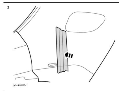
Apply a wide piece of tape to mark the rear hole for the net pocket.
