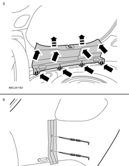
Remove the tailgate's sill panel by pulling it up until the four clips on the upper side and the eight catches at the lower edge release.
