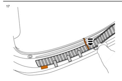
Allow the Bumper Protection to adhere to the Bumper Cover as indicated.
