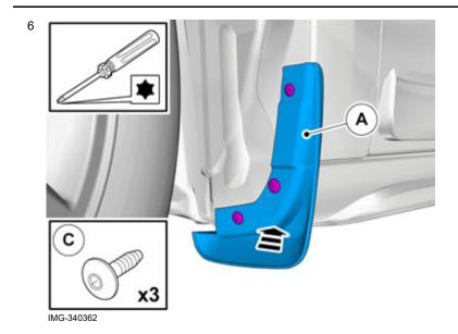
Install and screw the mudflap into place. Repeat the procedure on the other side.
