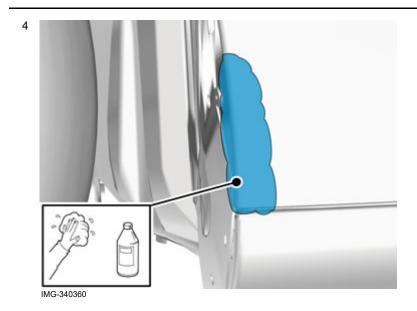
Clean the area where the protective tape is to be attached. Use: Isopropanol.
