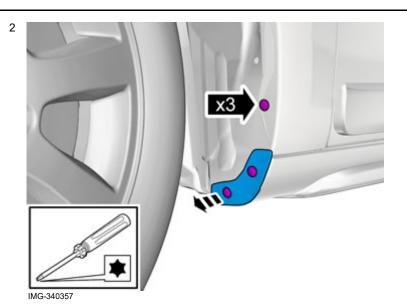
Remove the screws and flap. These will not be reused.
