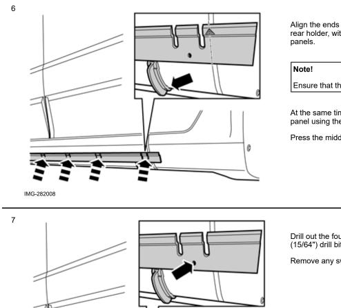
Ø 6mm (15/64") Align the ends of the markings that are at the rear edge on the rear holder, with the front part of the joint between the door sill
