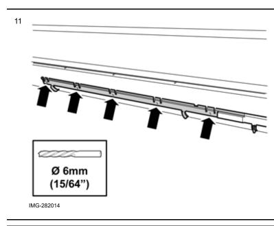
Drill out the five marked holes in the holder using a  $\emptyset$ 6 mm (15/64") drill bit.
