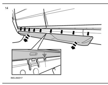
Hook the sill decor onto the holders. Start opposite the marking on the decor strip and cut-out, at the rear section of the front holder.
