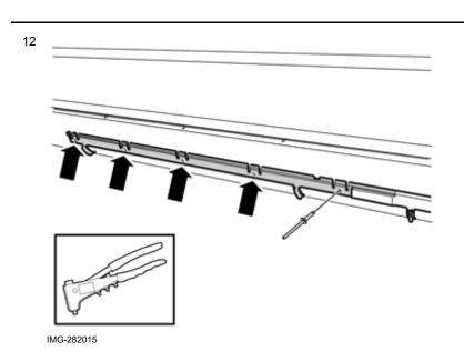
Take pop rivets from the kit. Rivet the holder to the door sill panel.
