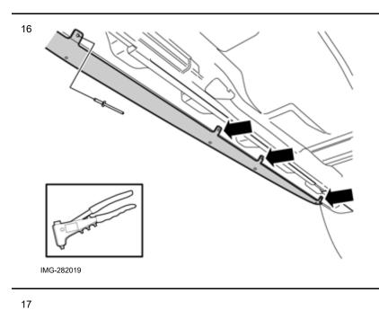
Rivet the mounting eyelets to the body using pop rivets.
