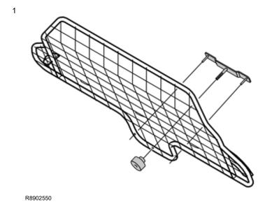
Remove the locking device from the cargo compartment net by unscrewing the knob and pulling it off.
