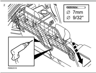
Lift in the cargo compartment net through the tailgate. Hang it on the backrest disc as illustrated. Check that the net is horizontal
