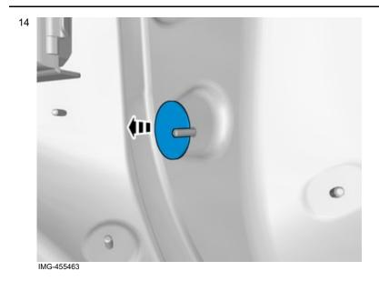
If the vehicle has a sealing plate, it should be removed.
