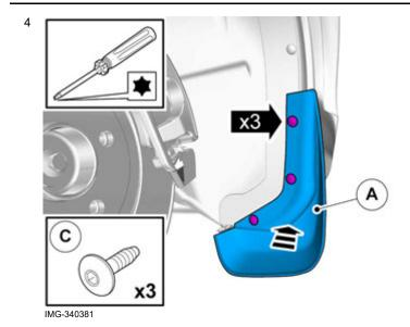
Install and screw the mudflap into place.
