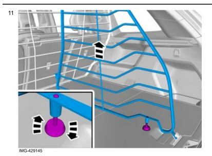
**Note!**Adjust the component indicated until no clearance or play is evident.
