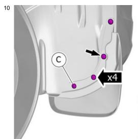
Install component that comes with the accessory kit. Tighten the bolts.
