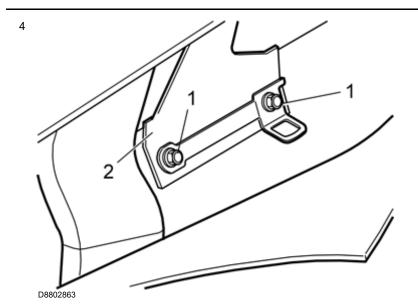
Remove the two screws from the bracket (2) on the tunnel (the screws will not be reused)
