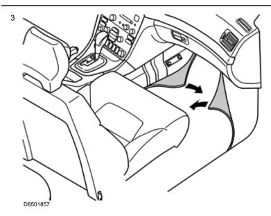
Push the floor carpet and insulation panel to one side.
