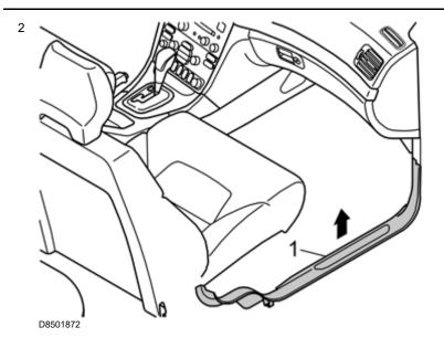
Remove the sill trim panel (1) by pulling upwards. Twist the front section inwards and unhook the rear section from the B-post panel.
