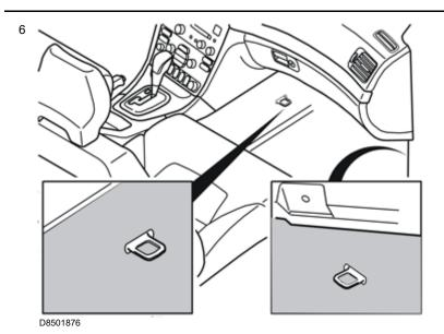
Fold the insulation panel and floor carpet back into position so that the mounting eyelets protrude through the stamped grooves in the floor carpet.
