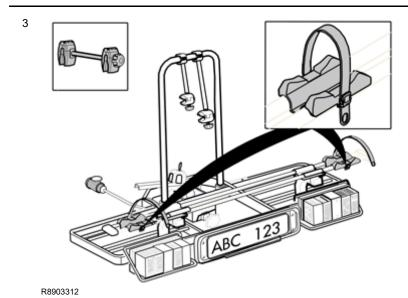
Installing the wheel strap and the bicycle frame holder
