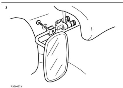
Screw the mirror into the mounting
