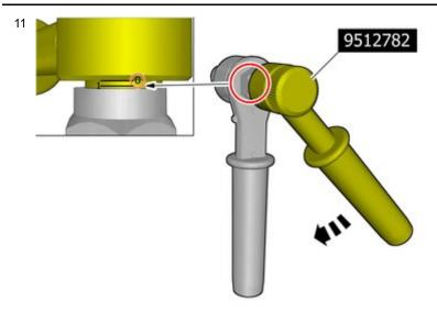
Use special tool: T9512782, Rivet nut tool
