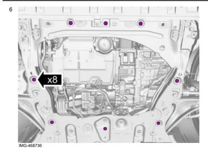
Remove the marked detail/details.
