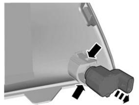
Carefully remove the sensor, it will not be reused.
