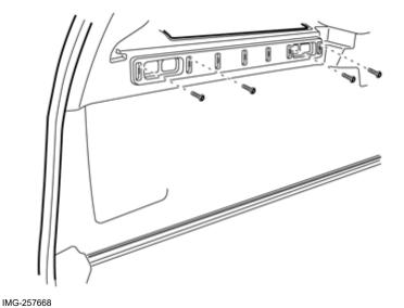
Align the rail, without the tape adhering, so that the four screws can be screwed into the side panel. The screws are self tapping and there may be some resistance when installing.
