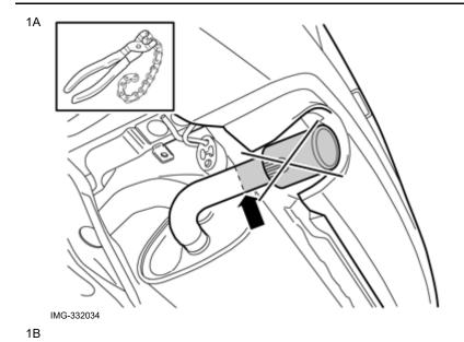
Cut off the pipe just in front of the joint using a pipe cutter.
