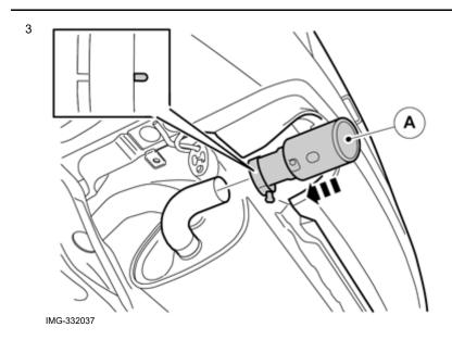
Install the end pipe. Slide it on so that the end of the slit covers the marking.
