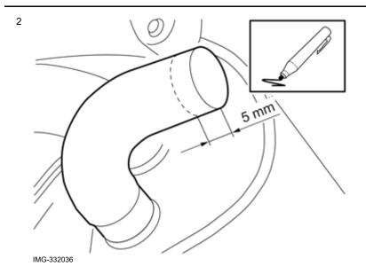
Mark 5 mm in on the cut pipe using a pen.
