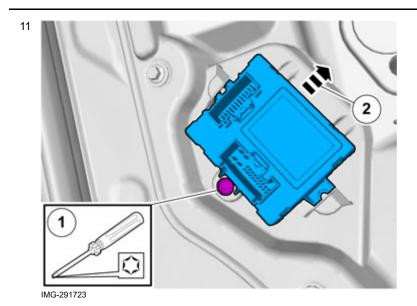
Remove the control module. This will not be reused.
