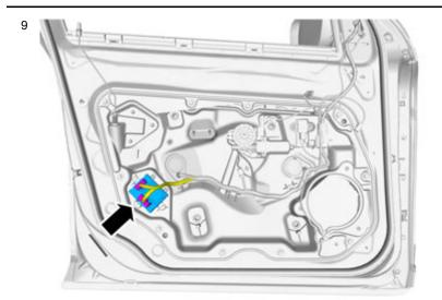
Replacement of the control module only applies to driver's door.
