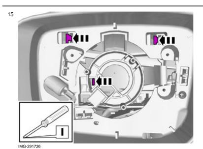
Release the three hooks and at the same time remove the cover
