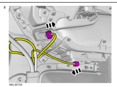
Disconnect the connectors and also any connectors for loudspeakers.
