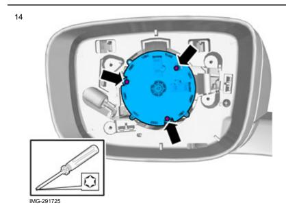
Remove the three screws, disconnect the connector and remove the motor unit.
