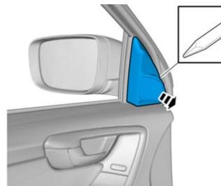
Remove the panel. Disconnect any connectors.
