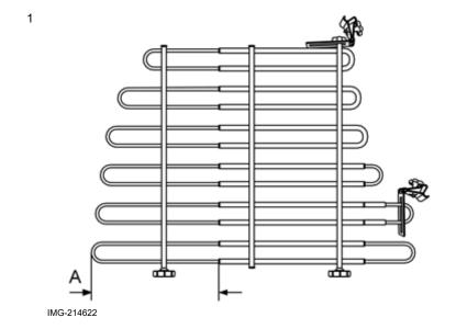
Before installing check the measurement at point A = 333 mm. Adjust as necessary.
