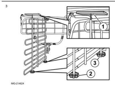
Adjust so that the cargo compartment wall is vertical and in the centre of the cargo compartment.
