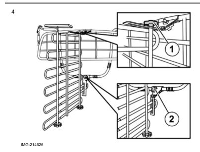
Tighten the knobs (1) and (2).
