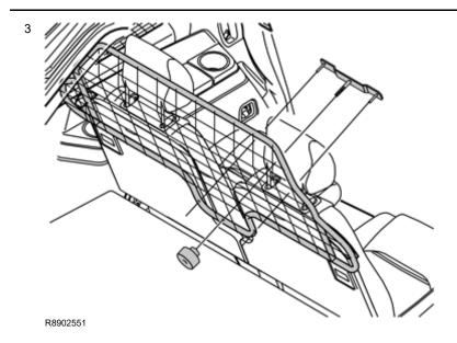
Take the striker plate and insert it from the front in the hole where it was disconnected
