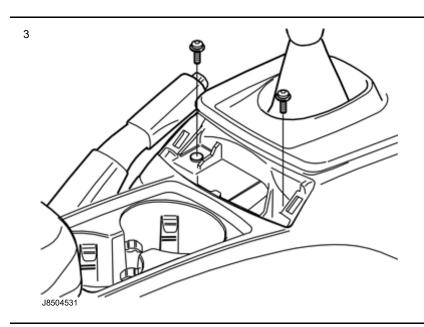
Remove the two screws holding the centre console at the rear edge.
