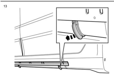
Twist loose the four mounting hooks from the holder.
