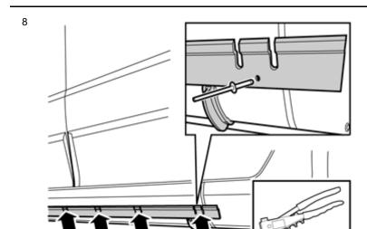
Take pop rivets from the kit. Rivet the holder to the door sill panel.
