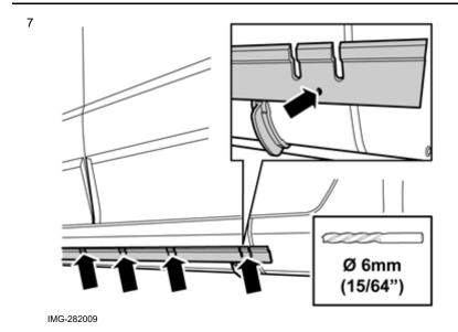
Drill out the four marked holes in the holder using a  $\emptyset$ 6 mm (15/64") drill bit.
