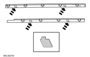
Press the pieces of tape onto the holders.
