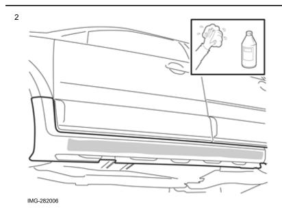
Clean the door sill panels using isopropanol where the decor panel's holder is to be positioned.
