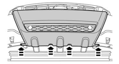
Install four new screws from the kit (similar to those removed) and tighten.
