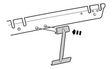
Take the two fixtures from the kit. Press them into the two holes in each end of the cradle, on the opposite side of the pieces of tape.
