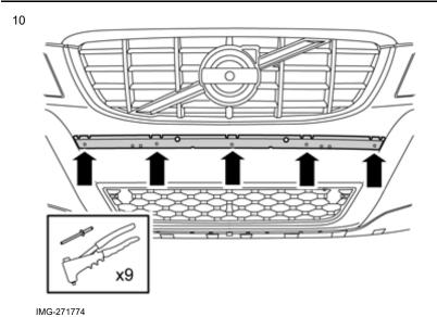
Pop rivet the cradle by starting to rivet from the centremost hole out towards the outermost, so that the cradle is securely attached all the way against the bumper cover.
