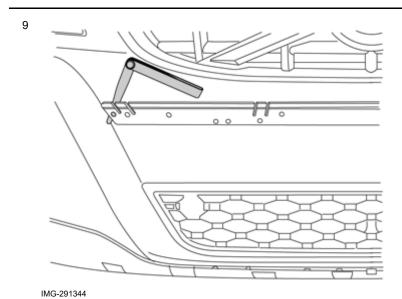
Take a feeler gauge and insert it behind the cradle at all drilled holes and remove all swarf.
