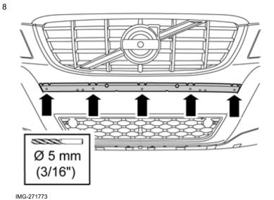
Take the Ø5 mm (3/16") drill bit. Drill through the pre-drilled holes on the cradle and through the bumper cover. Drill 10-15 mm (23/64 - 19/32") into the bumper cover to make room for the pop rivets.
