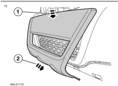
Place the panel on top of the cradle with the hooks opposite the corresponding cut-out in the panel, and angled 30 mm (1 3/16") at the lower edge.
