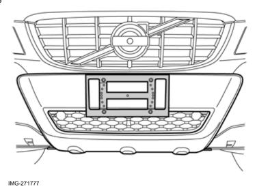
Install the number plate cradle with the new screws 4.8 x 14 mm (3/16 x 35/64 ") from the kit according to the markings.
