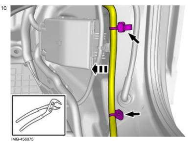
Remove the cable harness clips.
