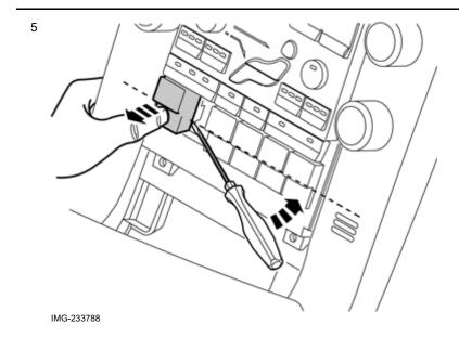
Carefully prize away the dummy button where the new switch shall be fitted. Use the thumb of your other hand to counterhold at the same time.
