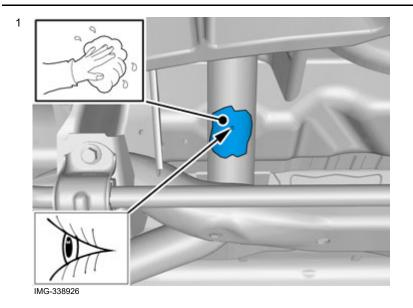
Locate the marking on the exhaust pipe.
