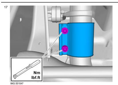
Tightening torque: M10 , 50 Nm
