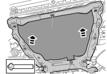
Cover the underneath of the engine with cardboard or similar, so that drilling swarf does not blow up into the engine compartment.
