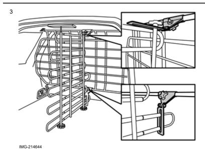
Position the cargo compartment wall with the clamps into the car.
