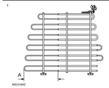
Before installing check the measurement at point A = 410 mm. Adjust as necessary.
