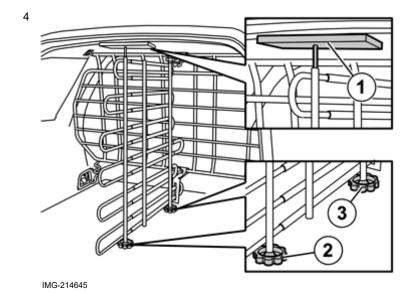
Adjust so that the cargo compartment wall is vertical and in the centre of the cargo compartment.
