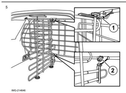
Tighten the knobs (1) and (2).
