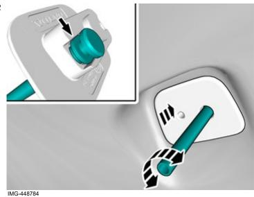
Turn marked detail while pushing the mounting to make the detail fit the mounting outlet
