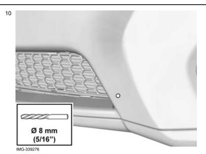
Drill the holes to Ø 8 mm (5/16 ").
