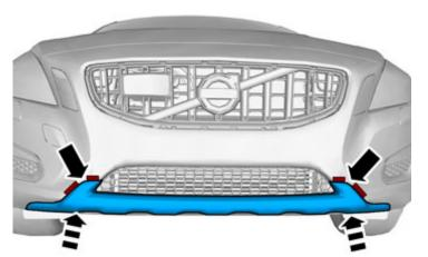
Centre the skid plate according to the markings made and press it so that the drilling templates secure on the inside.
