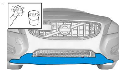
Wash the surfaces of the car that are to be covered by the skid plate.
