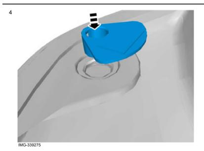
Take the drilling templates from the kit and press the drilling templates into the holes in the skid plate on both sides.
