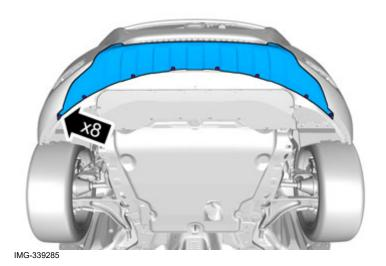
Tighten the skid plate below using screws from the kit. Start in the centre and work towards the sides.
