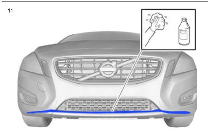
Clean using isopropanol where the tape on the skid plate was secured. Wipe dry.
