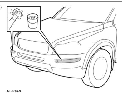
Clean the bumper cover where the decor strip is to be secured.
