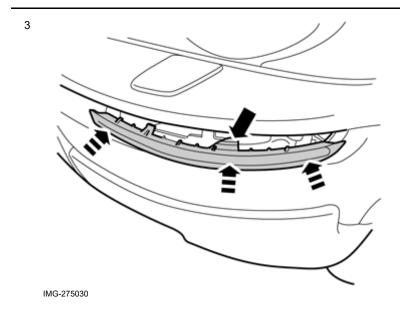
Align the decor panel in the cut-out and press it into place. Ensure that all hooks engage.
