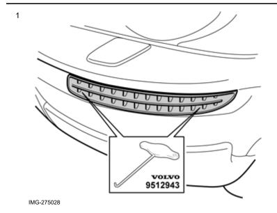
Carefully remove the bumper cover grilles on both sides by carefully pulling them off using tool part no. 9512943.
