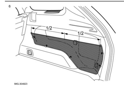
Measure out half the distance between the net pocket's eyelets and mark on the side panel, about the same height as the two eyelets.
