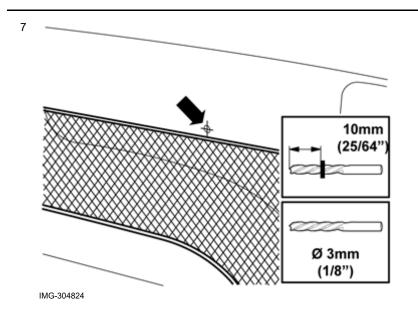
Drill the hole in the panel. Use drill stop.
