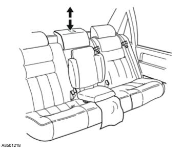
Adjust the head restraint so that it provides optimum protection for the child's head.
