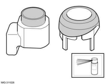
Paint the sensors and holders with the same color code as the decor trim around the fog lights' panels. Use paint recommended by Volvo. Paint max. two layers (1 layer base coat and 1 layer clear coat). Protect connections so that paint does not end up on the contact surfaces.
