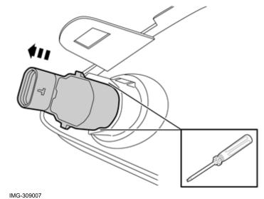
Remove the sensor by carefully prying up the catches and pulling it out.
