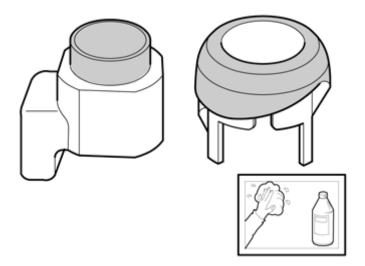
Clean the sensors and holders on the surface shown in the illustration. Use isopropanol and let dry.
