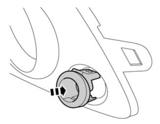
Take a new panel from the kit. Secure the sensor cradle in the new panel. Ensure that the catches engage.
