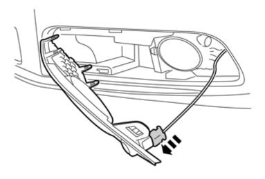
Plug in the connector to the sensor.
