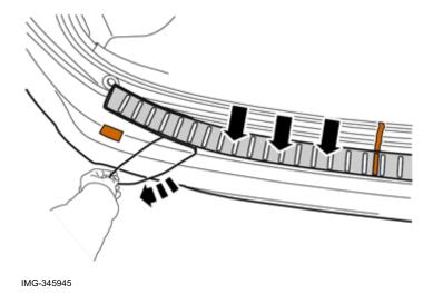
Pull off the rest of the transparent foil and press by hand on the Bumper protection to make it cling to the Bumper Cover.
