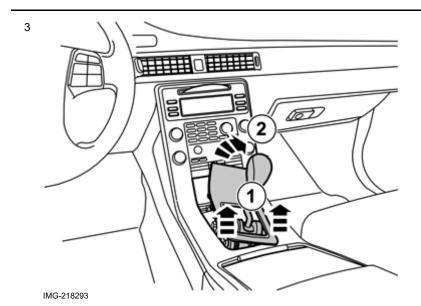
Twist / remove the panel, so that the row with switches/dummy buttons is accessible.
