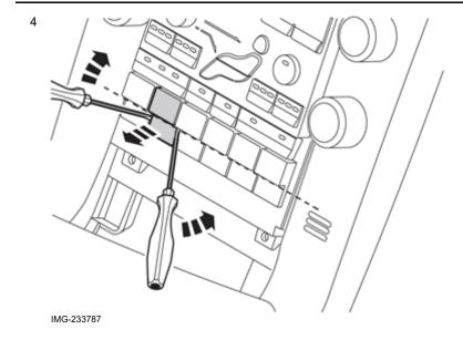
The new switch must be fitted in the first available button location seen from the steering wheel.
