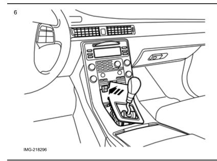
Install the new switch from the kit, and any dummy button.
