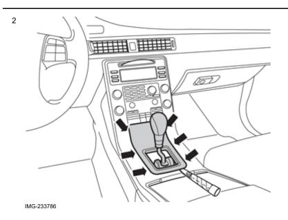
Carefully prize away the panel around the gear selector lever using a weatherstrip tool. It is secured along the longitudinal sides with six catches. Start prizing in the rear edge of the panel.
