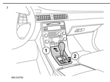
Reinstall the panel around the gear selector lever
