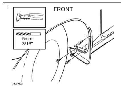
Clean around the screw holes in the rear edge of the wing liner
