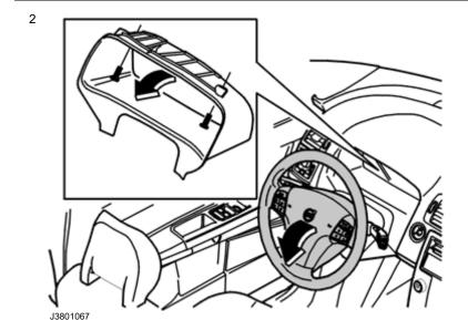
Adjust the steering wheel to the outermost and lowermost position.
