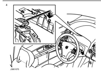
Take the new instrument panel and connect the connector.
