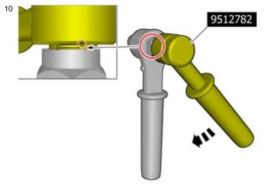
Use special tool: T9512782, Rivet nut tool
