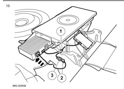
Take the fibre optic adapter cable (1) from the kit and connect both the male connectors to the Subwoofer, respectively, Sirius unit.
