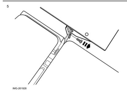
Remove the screw from the left-hand mounting.
