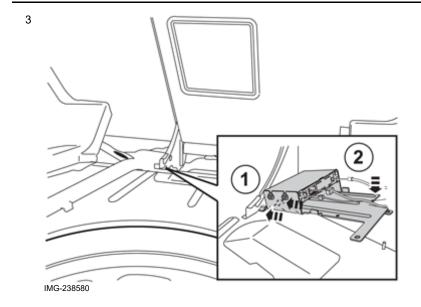
Insert the two legs of the bracket in the corresponding recesses in the backrest bracket and lower it over the retaining pin in the floor.
