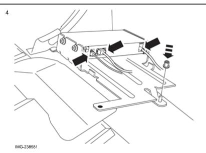
Secure the bracket using a plastic nut from the kit.
