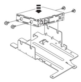
Install the Sirius unit on the bracket with four screws and washers from the kit.
