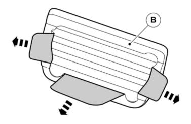
Hold the pedal protector as illustrated and fold out the three tabs.
