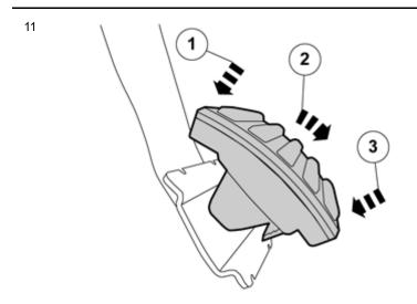
Hook the protector on at the upper edge, at the same time hold the tabs and pull downwards.
