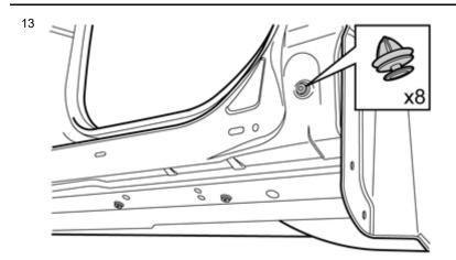
Remove all clips (8 pcs on each side) from the door sill, and in the front and rear wings, and replace them with new ones.
