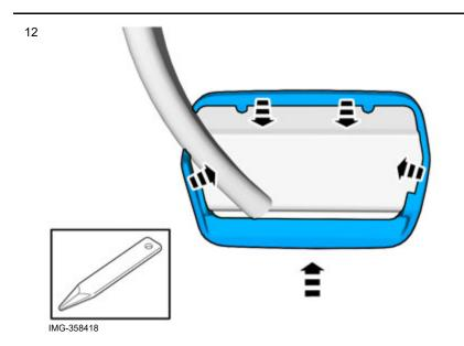
Press the pedal rubber towards the pedal and at the same time fold the pedal rubber's profile over the pedal using a straightening tool.
