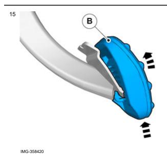
Hook the pedal rubber onto the pedal at the lower edge and pull the pedal rubber upward.
