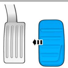
Hook the pedal rubber onto the long side of the accelerator pedal.
