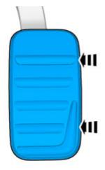
Press the pedal rubber towards the pedal and at the same time fold the pedal rubber's profile over the pedal using a straightening tool.
