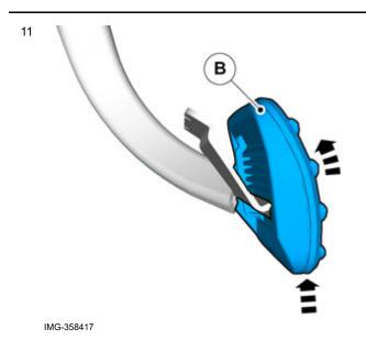
Hook the pedal rubber onto the pedal at the lower edge and pull the pedal rubber upward.
