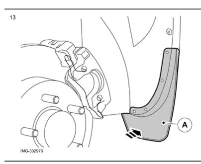
Fold the inner wing back and install the mudflap.
