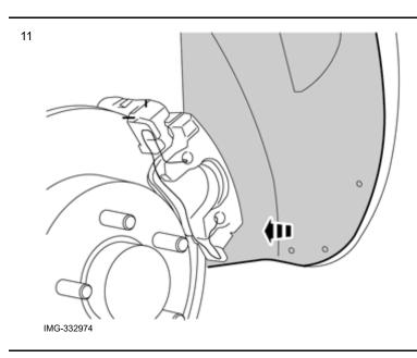
Fold the wing liner out of the way.
