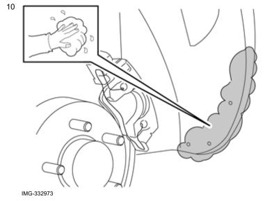
Clean the area where the mudflap is to be positioned.
