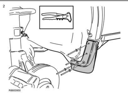
Install the mudflap and rivet it to the wing liner and rear edge of the front wing.
