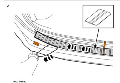
Pull off the rest of the transparent foil and press by hand on the Bumper protection to make it cling to the Bumper Cover.
