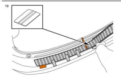
Use suitable tool to squeeze out any trapped air bubbles.
