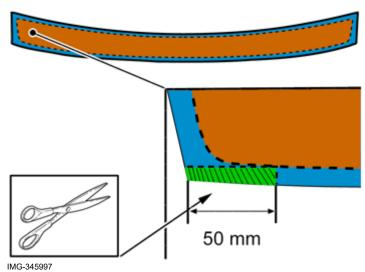
Center the Bumper Cover, using the tape marks and the values in the graphic.
