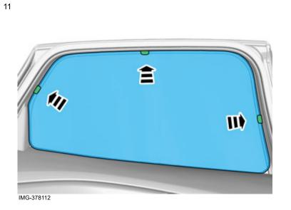
**Note!** The part must be bent during installation.
